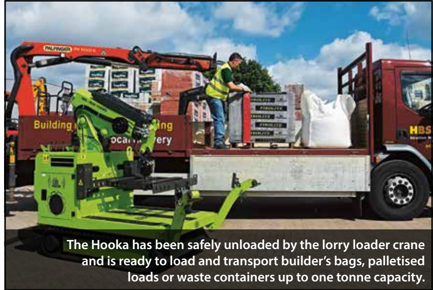
The Hooka is short enough to be slewed across the width of the truck loadbed, thereby only using 1m of platform length.
