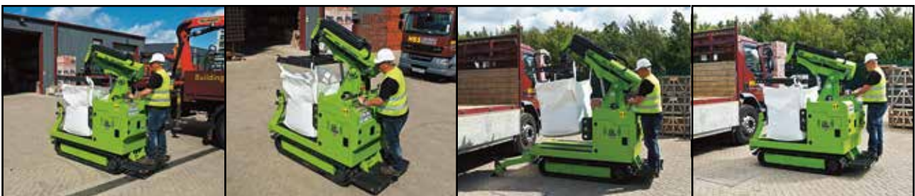
Using a bag spreader attachment, with full rotation option – the loaded builder's bag is lifted off the truck loadbed; the bag is then teleboomed in, while the front-mounted jack leg stabilisers remain down; the loaded bag is safely located on the Hooka's loadbed platform and the telescopic crane stowed for transit mode; and the Hooka is now ready to deliver – or collect – bags from the far reaches of any site.
